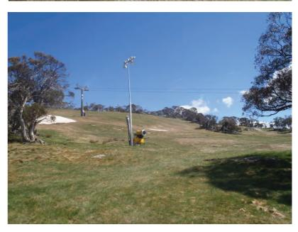
Figure 15: Existing light pole and fan gun to be removed and re-located (F2)
